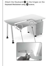
(Note: When the keyboard surface cannot be on the same level with the monitor surface, you can release the bolts on 2 arms of keyboard mechanism for pulling down or lifting up, then fasten the bolts tightly).
